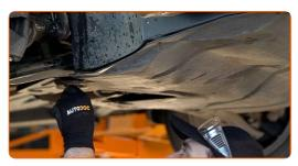
Remove the lower sound insulation.
