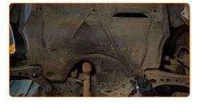
Remove the lower sound insulation.
