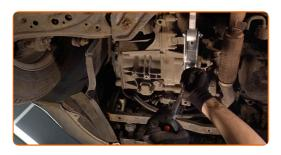
13.1 Tighten the engine mount fastening bolts.
