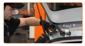
Release the circlip connecting the gas strut to the boot lid. Use a flat screwdriver.
