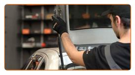
5 Install the new boot lid gas strut.
