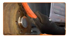
Treat the contacting surface. Use copper grease.
