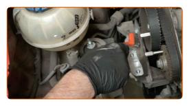
Unscrew the engine mount fasteners. Use a drive socket #16. Use a ratchet wrench.
