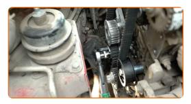
Remove the camshaft gear locking tool.
