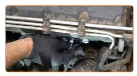
Tighten the glow plugs. Use the spark plug socket #10. Use a torque wrench. Tighten it to 15 nm torque.
