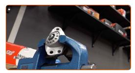
Screw the shock strut piston rod upper fastening. Use a combination spanner #17. Use an adjustable wrench. Use a torque wrench. Tighten it to 25 Nm torque.
