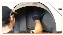
Install and tighten the wheel arch cover fasteners. Use Torx T25.
