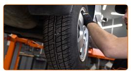
Unscrew and remove the wheel arch cover fasteners. Use Torx T25.
