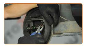
Pull both brake shoes with the adjuster from the working brake cylinder, avoiding damage to the boots.
