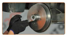
10 Remove the brake drum.
