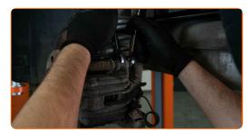
11 Remove the brake caliper.
