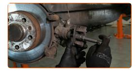
Treat the back side of the new brake pads. Treat the brake caliper bracket where it contacts the brake pads. Use anti-squeal paste.
