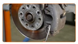
11 Remove the brake caliper.
