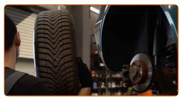
Clean the area where the brake hose is connected to the caliper, and the guide pins area. Use a wire brush. Use a brake cleaner.
