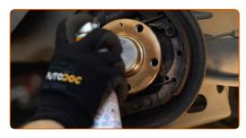
Install the brake drum and fasten it.
