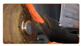
Treat the contacting surface. Use copper grease.
