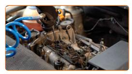
Unscrew the spark plugs. Use the spark plug socket #16. Use a ratchet wrench.
