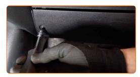
Pry up, carefully release from the fasteners and remove the side trim panel on the passenger side.
