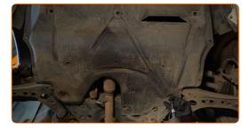
Remove the lower sound insulation.
