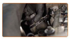
Screw the cap. Use a drive socket #36. Use a torque wrench. Tighten it to 25 Nm torque.
