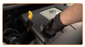
Pour oil into the engine through the filler. Required amount of oil: 3.3 l.
