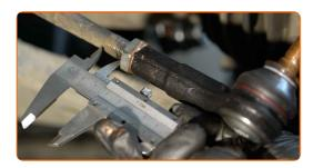
Screw on the fastening nut that connects the tie rod end to the steering knuckle. Use a drive socket #19. Use a ratchet wrench.
