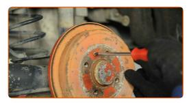
Remove the brake drum.
