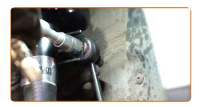
Tighten the fastener connecting the stabilizer link to the stabilizer bar. Use a combination spanner #16. Use Torx T30. Use a torque wrench. Tighten it to 40 Nm torque.
