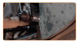
Tighten the fastener connecting the stabilizer link to the shock strut. Use a drive socket #16. Use a torque wrench. Tighten it to 40 Nm torque.
