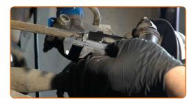
Loosen the lock nut securing the tie rod end to the tie rod. Use a combination spanner #22.
