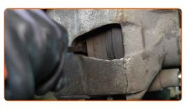
Remove the brake caliper.
