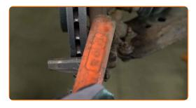
Remove the brake pads. Use a crowbar.
