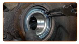
Dismantle the inner bearing race that is remaining on the hub. Bush and bearing driver set. Use a bearing separator.
