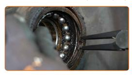
Press out the wheel hub bearing. Use a bearing driver tool set.
