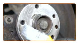
Install the brake disc.
