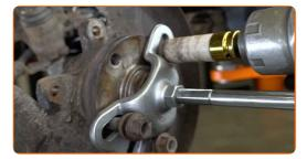
Clean the wheel hub bearing retaining ring. Use a wire brush. Use WD-40 spray.
