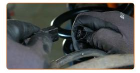
Clean the brake caliper retaining spring. Use a wire brush. Use a brake cleaner.
