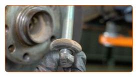
Remove the spring washer with a reluctor ring.
