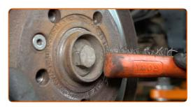
Unscrew the brake disc fastening. Use HEX No.H6. Use a ratchet wrench.
