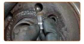
Remove the brake disc.
