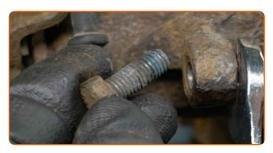
Remove the brake caliper. Use a crowbar.
