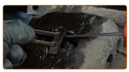
Clean the brake caliper fasteners. Use a wire brush. Use a brake cleaner.
