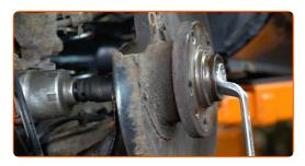
Remove the fastening bolt.
