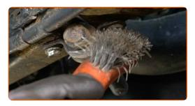
Unscrew the fasteners that connect the sway bar to the suspension arms. Use a drive socket #13. Use a ratchet wrench.
