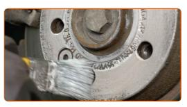
Clean the brake disk surface. Use a brake cleaner.
