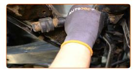
Tighten the fasteners that connect the sway bar to the suspension arms. Use a drive socket #13. Use a torque wrench. Tighten it to 35 Nm torque.
