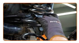
Remove the rubber mounts of the spring.
