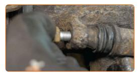
Tighten the brake caliper fasteners. Use a combination spanner #15. Use a drive socket #13. Use a torque wrench. Tighten it to 35 Nm torque.
