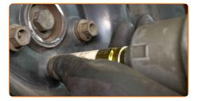
Lower the car and working in a cross order, tighten the wheel bolts. Use wheel impact socket #19. Use a torque wrench. Tighten it to 170 Nm torque.
