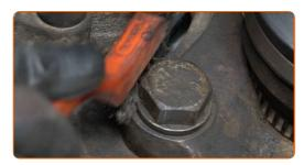
Unscrew the caliper bracket fastening. Use a drive socket #27. Use a ratchet wrench.
