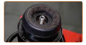
Tighten the shock strut piston rod nut. Use a 21-mm strut nut socket. Use HEX No.H7. Use a torque wrench. Tighten it to 60 nm torque.
