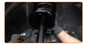
Screw in the top fasteners of the suspension strut mount. Do not tighten it.
