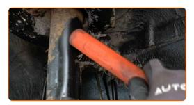
Unscrew the fastener connecting the stabilizer link to the shock strut. Use a combination spanner #16. Use a drive socket #19. Use a ratchet wrench.
