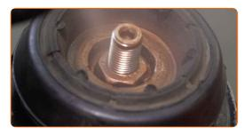
Remove the assembled shock strut.
