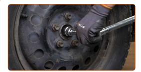
Tighten the wheel bolts using a criss-cross pattern. Use wheel impact socket #19. Use a torque wrench. Tighten it to 170 Nm torque.
