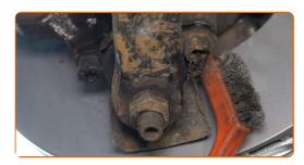
Unscrew the ball joint fasteners from the steering knuckle. Use HEX No.H8. Use a ratchet wrench.
