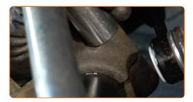
76 Connect the ABS sensor wiring.
