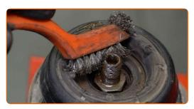
Remove the strut piston rod nut. Use a 21-mm strut nut socket. Use HEX No.H7. Use a ratchet wrench.
