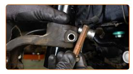
Screw in the lower fastener of the shock strut. Use a drive socket #18. Use a ratchet wrench.
