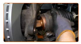
65 Connect the ball joint to the steering knuckle.
