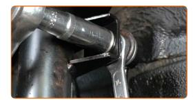
Tighten the lower fasteners of the suspension strut. Use a drive socket #18. Use a torque wrench. Tighten it to 110 Nm torque.
