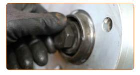
Screw in the fastener of the CV axle. Use a drive socket #27. Use a ratchet wrench.
