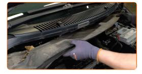
Clean the upper fastener of the suspension strut mount. Use a wire brush. Use WD-40 spray.
