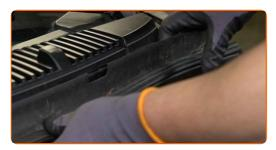
Unscrew the plastic panel fasteners. Use a drive socket #10. Use a ratchet wrench.
