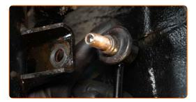
Disconnect the ABS sensor wiring.
