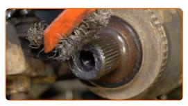
Treat the splines of the driveshaft CV joint. Use copper grease.
