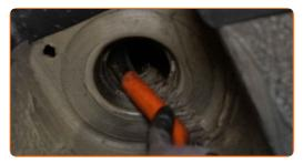
Clean the fasteners that connect the ball joint to the steering knuckle. Use a wire brush. Use WD-40 spray.
