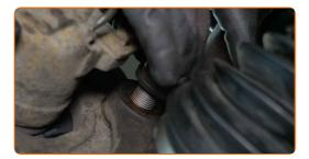
Tighten the brake caliper bracket fasteners. Use a drive socket #27. Use a torque wrench. Tighten it to 200 nm torque.
