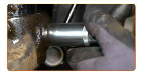
Remove the fastening bolt.
