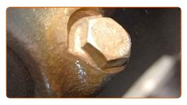
Treat the fastener that connects the sway bar link to the suspension strut. Use copper grease.
