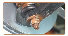
Treat the fastener that connects the suspension strut to the steering knuckle. Use copper grease.
