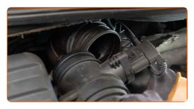
Cover the air intake hose with a microfibre towel to prevent dust and dirt from getting into the system.
