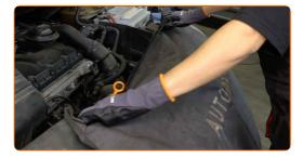
Undo the fastening screws of the air filter cover. Use a Phillips screwdriver.
