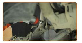
Remove the fastening bolt.
