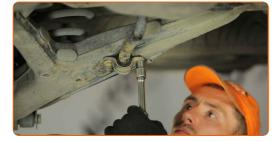
Treat the fasteners of the stabilizer bush brackets. Use copper grease.
