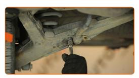
Remove the stabilizer bush brackets. Use a flat screwdriver.
