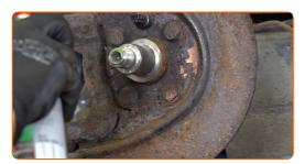
Apply special grease to the bearing assembly mounting seat.
