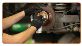
24 Install the brake disc.
