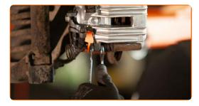
Remove the brake caliper.
