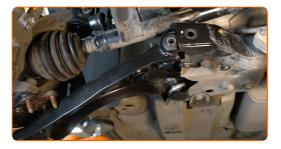
Replacement: front lower arm – SEAT Toledo IV Hatchback (KG3). Tip:
