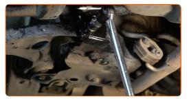
Unscrew the rear fastener connecting the control arm to the subframe. Use a combination spanner #18. Use a drive socket #18. Use a tap wrench.
