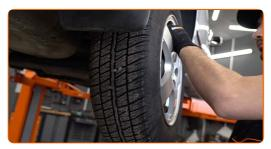
6 Unscrew and remove the wheel arch cover fasteners. Use Torx T25.
