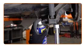
Unscrew the lower fastener of the shock absorber. Use a combination spanner #16. Use a drive socket #16. Use a ratchet wrench.
