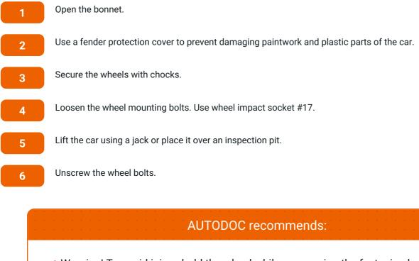
• Warning! To avoid injury, hold the wheel while unscrewing the fastening bolts. SEAT Toledo IV Hatchback (KG3)
