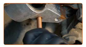
Screw the rear fastener connecting the control arm to the subframe. Use a combination spanner #16. Use a drive socket #16. Use a ratchet wrench.
