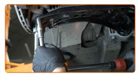
Tighten the rear fastener connecting the arm to the body subframe. Use a drive socket #16. Use a torque wrench. Tighten it to 50 Nm torque.+90°
