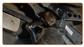
Remove the support from under the arm.
