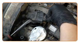
Replacement: spark plugs – SEAT Toledo III (5P2). Tip from AUTODOC:
