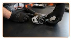
Screw the shock strut piston rod upper fastening. Use a combination spanner #16. Use an adjustable wrench. Use a torque wrench. Tighten it to 25 Nm torque.
