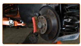
Treat the contacting surface. Use copper grease.
