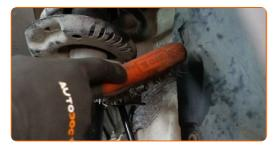
Unscrew the fastener connecting the stabilizer link to the shock strut. Use a drive socket #19. Use a ratchet wrench.
