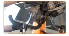
Clean the clamps of the CV joint boot. Use a wire brush. Use WD-40 spray.
