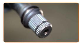
Pack the CV joint with the grease supplied in the kit.
