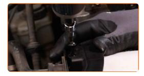
Reinstall the air filter cover. Fasten it.
