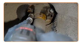
10 Remove the fastening bolt.
