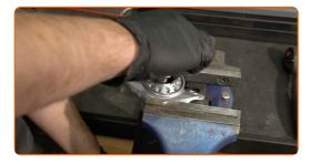
Tighten the shock absorber rod nut. Use a drive socket #16. Use a shock absorber socket DD№6. Use a torque wrench. Tighten it to 25 nm torque.
