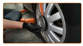
Unscrew the hub lock nut. Use 1-3/16" drive 12-point socket.
