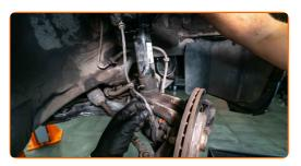
Unscrew the fastener connecting the drive shaft to the wheel hub. Use 1-3/16" drive 12-point socket.
