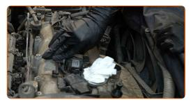
Tighten the chassis (ground) terminal of the ignition coils. Use a drive socket #10. Use a ratchet wrench.
