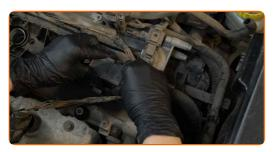
Install the ignition coils to the spark plug wells. Make sure you hear a click indicating that it is locked in place.
