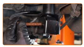
Screw in the lower fastener of the shock absorber. Use a combination spanner #16 (2 pieces). Use a ratchet wrench.
