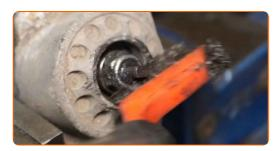
Unscrew the fastener of the shock absorber piston rod. Use a drive socket #17. Use a shock absorber socket #DD5.2. Use a ratchet wrench.
