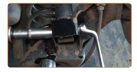
Remove the fastening bolt.
