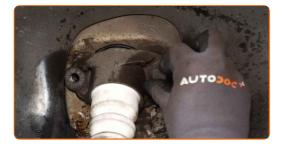
Screw in the shock absorber mount fasteners. Use a drive socket #16. Use a ratchet wrench.
