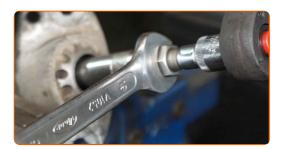
Remove the shock absorber mount, dust boot, and bump stop.
