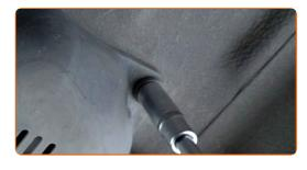
Remove the oxygen sensor housing cover.
