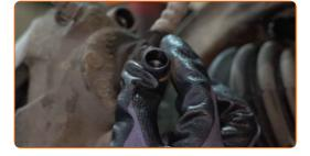
Unscrew the brake caliper fasteners. Use HEX No.H7. Use a ratchet wrench.
