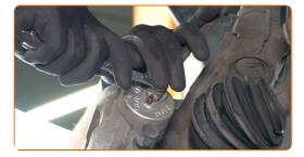
Loosen the fastener connecting the brake pipe to the brake hose. Use a combination spanner #11.
