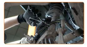
Connect the brake bleeder kit to the brake bleeder screw.
