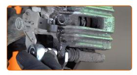
Remove the brake caliper. Use a crowbar.
