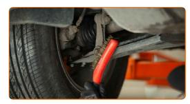
Unscrew the fasteners connecting the stabiliser link to the stabiliser bar and to the suspension control arm. Use a combination spanner #16. Use a torque wrench.
