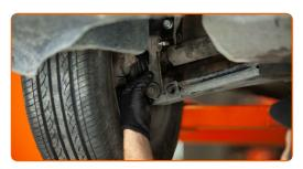
Clean all joints of the stabiliser link. Use a wire brush. Treat all joints of the stabiliser link. Use WD-40 spray.
