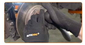
15 Remove the brake disc.
