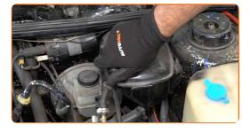
Remove the fender protection cover.
