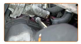
Remove the thermostat housing.
