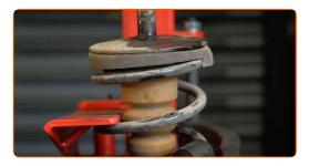
Remove the strut piston rod nut. Use a combination spanner #17. Use a shock absorber socket #DD5,2. Use a ratchet wrench.
