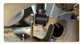
Tighten the lower fastening of the shock absorber. Use a combination spanner #17. Use a drive socket #17. Use a torque wrench. Tighten it to 70 nm torque.
