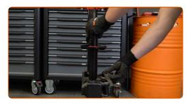
Install the spring on the shock absorber.
