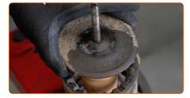
Release the coil spring.
