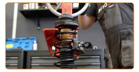
Remove the assembled shock strut.
