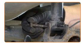
18 Remove the suspension strut.
